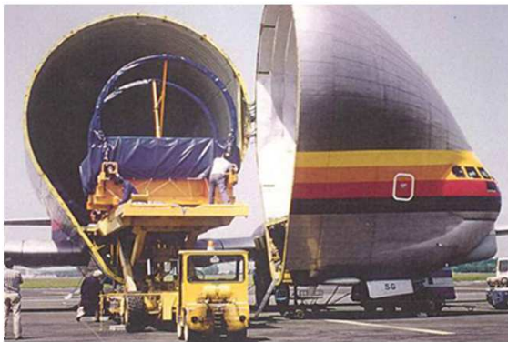
July 1 st , 1985 Nantes dispatches the first A320 centre wing box
