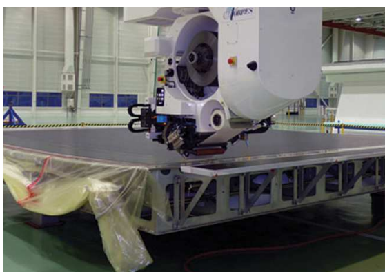
December 4 th , 2009 Lay-up of the first composite plies of the A350 XWB centre wing box
